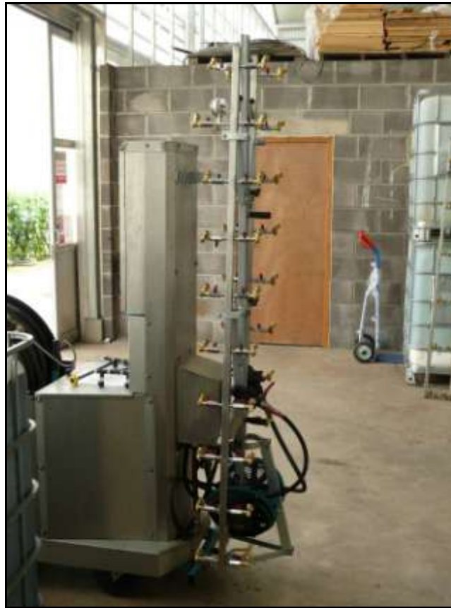
Figure ii. New booms fitted to the robotic sprayer:
